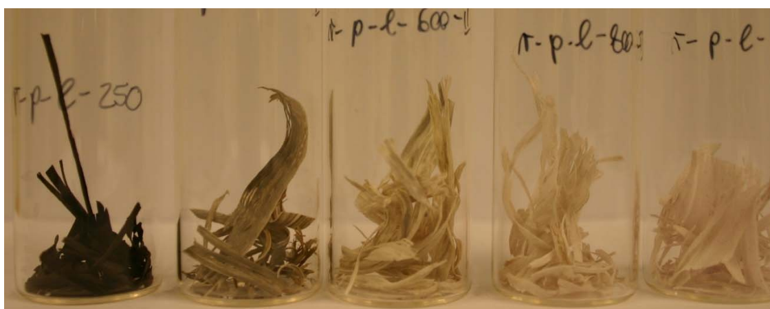
Fig. 20: remains of the leaves of phragmites from 250°C on the left to 1000°C on the right (Ø of vessels = 30 mm; photo © D. Fritzsch).
