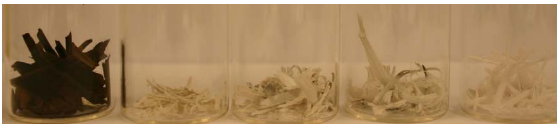
Fig. 21: remains of the stems of phragmites from 250°C on the left to 1000°C on the right (Ø of vessels = 30 mm; photo © D. Fritzscht).
